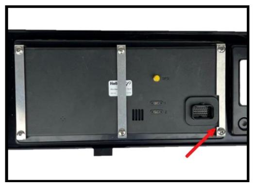
Install bracket with notch on right side of Holley 12.3" as shown above.
