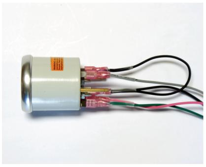
The Water Temperature Gauge Will have 4 Wires going to it, first will be a Green Temperature Wire to the Signal Tab, Second will be a 12 Volt + Pink Wire going to the 12V+ Tab, Third will be a Gray Gauge Light Wire for the gauge Lights going to the Light Tab, fourth will be the Black Wire which is a ground for the gauge. In Bag 5204 You will need to use the jumper wire and connect it to the gauge light ground and connect the black wire to the secondary pin on the jumper wire.
