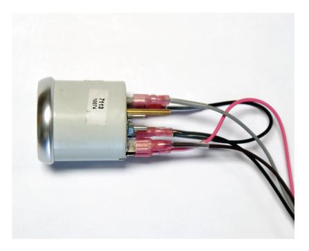
The Fuel Gauge Will have 4 Wires going to it, first will be a Brown Fuel Gauge Wire to the Signal Tab, Second will be a 12 Volt + Pink Wire going to the 12V+ Tab, Third will be a Gray Gauge Light Wire for the gauge Lights going to the Light Tab, fourth will be the Black Wire which is a ground for the gauge. In Bag 5204 You will need to use the jumper wire and connect it to the gauge light ground and connect the black wire to the secondary pin on the jumper wire.
