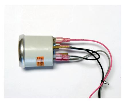
The Volt Gauge Will have 3 Wires going to it, first will be a 12 Volt + Pink Wire going to the 12V+ Tab, Second will be a Gray Gauge Light Wire for the gauge Lights going to the Light Tab, Third will be the Black Wire which is a ground for the gauge. In Bag 5204 You will need to use the jumper wire and connect it to the gauge light ground and connect the black wire to the secondary pin on the jumper wire.
