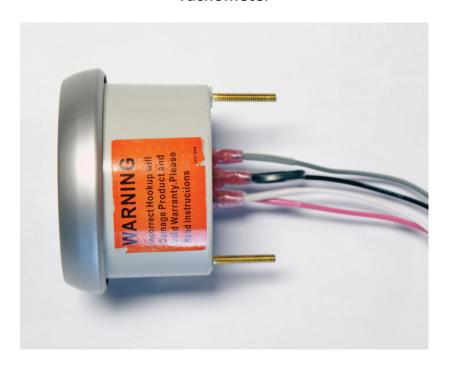
The Tachometer will have 4 Wires going to it, first will be a White Coil Wire to the Signal Tab, Second will be a 12 Volt + Pink Wire going to the 12V+ Tab, Third will be a Gray Gauge Light Wire for the gauge Lights going to the Light Tab, fourth will be the Black Wire which is a ground and will attach to the Ground Tab.
