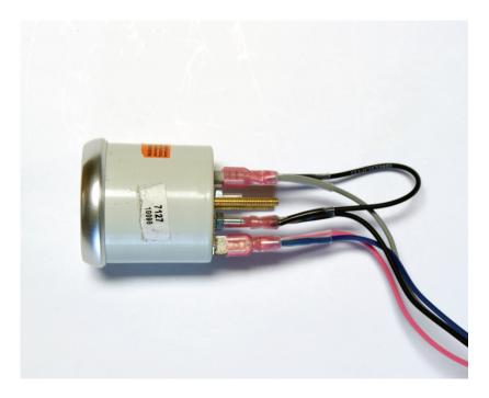
The Oil Pressure Gauge Will have 4 Wires going to it, first will be a Blue Oil Pressure Wire to the Signal Tab, Second will be a 12 Volt + Pink Wire going to the 12V+ Tab, Third will be a Gray Gauge Light Wire for the gauge Lights going to the Light Tab, fourth will be the Black Wire which is a ground for the gauge. In Bag 5204 You will need to use the jumper wire and connect it to the gauge light ground and connect the black wire to the secondary pin on the jumper wire.
