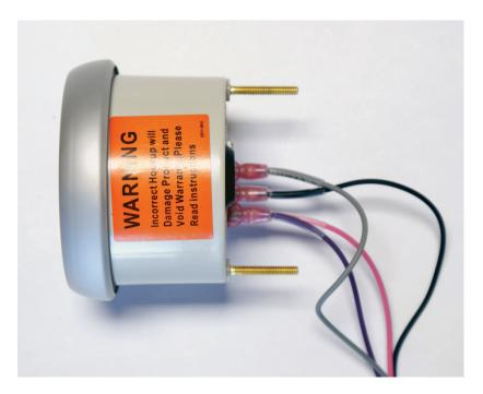
The Speedometer will have 4 Wires going to it, first will be a Purple VSS Wire to the Signal Tab, Second will be a 12 Volt + Pink Wire going to the 12V+ Tab, Third will be a Gray Gauge Light Wire for the gauge Lights going to the Light Tab, fourth will be the Black Wire which is a ground and will attach to the Ground Tab.
