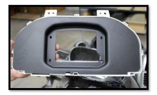
Step 11: Re-attach the hood in the dash carrier, without the glass lens.
