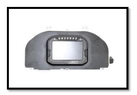
Step 10: Attach Classic Dash panel to white back housing using included attachment screw kit.
