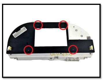
Step 8: Remove the template and clean off white back piece of any excess debris.
