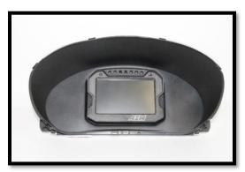
Step 12: Place Classic Dash panel and AEM assembly back into dash carrier.
