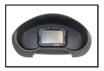
Step 12: Place Classic Dash panel and AEM assembly back into dash carrier.
