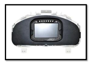
Step 10: Attach Classic Dash panel to white back housing using included attachment screw kit.
