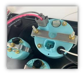
The GPS Plug-and-Play Antenna (included) plugs directly into the back of the speedometer. The black and white wires shown on the back of the speedometer are for TRIP / RESET. Install push button switch (included) between these two wires.
