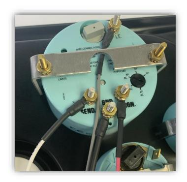
The black knob on the right side on the back of the gauge MUST be set to the correct cylinder number of your engine in order for the tachometer to function properly.
