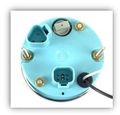
The speedometer will have a triangular plug that connects all of the necessary wires to the back of the gauge.
