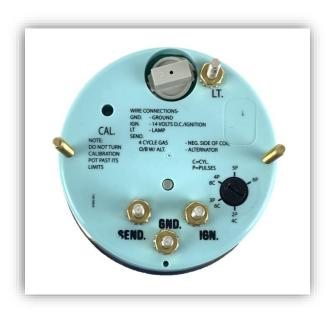
The tachometer will have 4 wires connecting to it:
