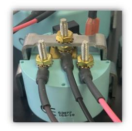
The fuel level gauge will have 4 wires connecting to it:
