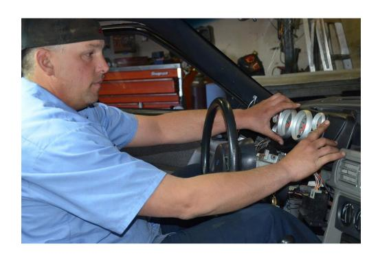
Trial fit the new Classic Dash panel and trim it if required. Pull the panel towards you and locate the factory loom plugs. Squeeze the tangs together and insert the male end into the female receptor on the Classic Dash loom. Make sure both plugs are secure.
