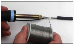
3. Apply heat to the splice from the soldering iron./pen and feed a small diameter, quality 50/50 solder to the iron and let the molten solder absorb into the connection.
