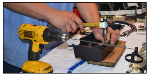
Prior to drilling the 5/32" holes for the warning lights use a punch and mark where the hole is to be placed. Cement the lights in place.
