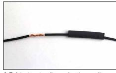
2. Twist wires together and make sure the sleeve is kept away from any heat source
