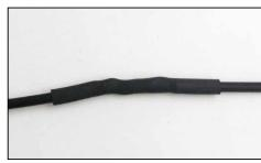
4. Side the tubing over the connection and apply heat from a heat gun or lighter so it shrinks the sleeve and seals the joint.
