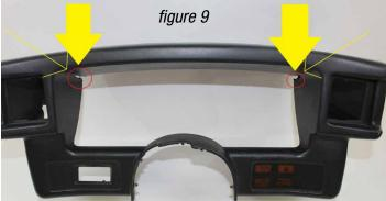
Some customers may need to make small incisions to their dash bezel to make installation of our dash panel easier. A Dremel tool or a reciprocating saw are recommended to make these cuts.
