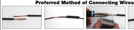
1. Strip wires 1/2" to 3/4" and lay opposing as shown. Slide sleeve over one wire.
